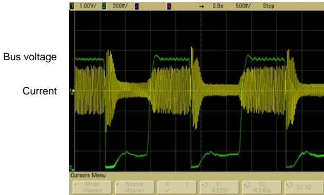
Fig. 2 The inverter realizes stable control of current and voltage and will not trigger under any acceleration/deceleration condition as well as stable operation condition
